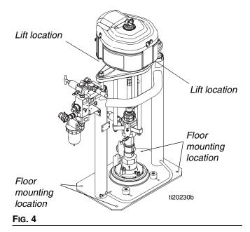
Attach a lifting sling at the proper lift spots. Lift off the pallet using a crane or a forklift.
